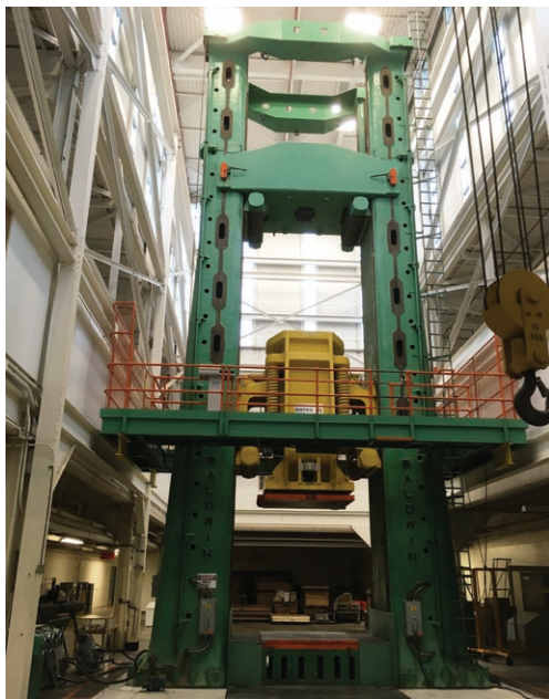
Reclamation's Compression Strength Test Press at the Reclamation Technical Services Center in Denver.
